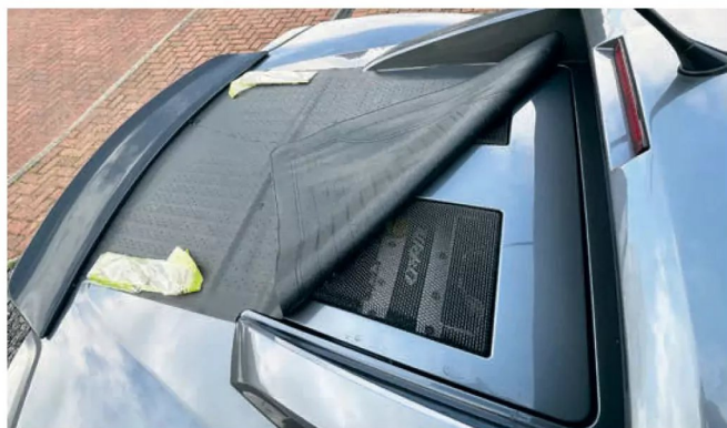
Mid-engined with vents in the engine 'bonnet', rainwater can find its way to the coil pack that sits right on top of the engine, so an aftermarket rubber cover was purchased.
