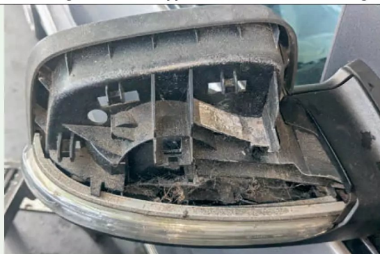
The old failed LED lamp needed to be removed and so the door mirror casing had to be unclipped to allow access to the fixings.
