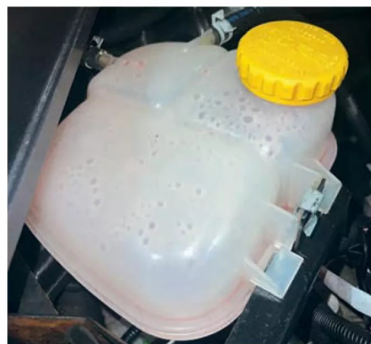
The expansion tank suffers from UV exposure, cracking the plastic – febi offer these in their catalogue, however this was recently replaced.
