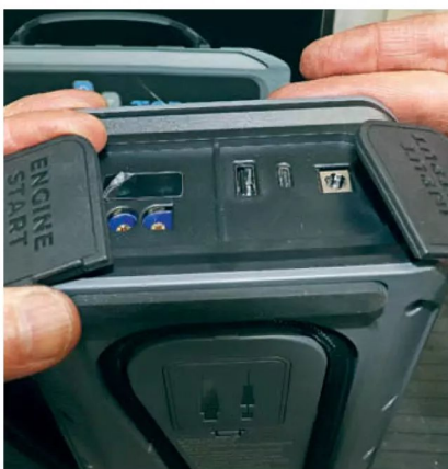
Ports on the side of the V2200Air look obvious, but only the USB-A and round port are for recharging another device, whereas the USB-C is for recharging the on-board battery.
