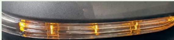
The old failed LED lamp needed to be removed and so the door mirror casing had to be unclipped to allow access to the fixings.
