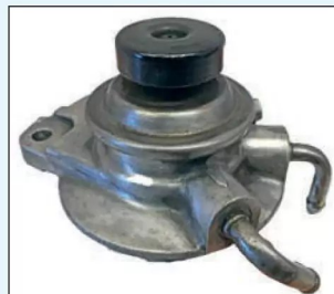
The fuel primer which is part of the fuel filter housing may be allowing air into the system.
