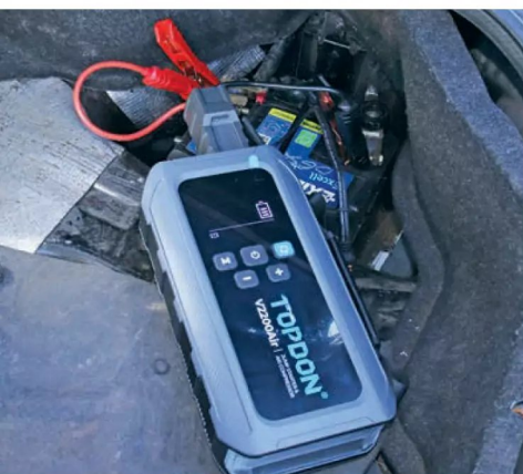
Jump-starting Rob's MX-5 where the vehicle battery needed a boost, saw it rise to 14V after initially connecting the V2200Air. A twist of the ignition key fired the engine to life.
