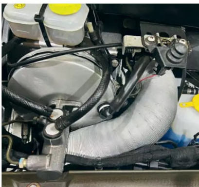
The VX220 never came with a pollen filter – this aluminium tubing feeds unfiltered air directly into the cabin!
